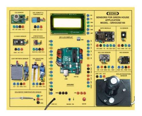
This trainer has been designed with a view to provide practical and experimental knowledge Sensors programing for IoT based Green House Application with Arduino IOT Board.
